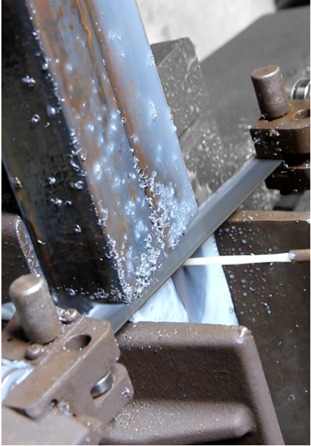
Step 2: CUTTING OF WORKPIECE (FLAT ANCHOR HEAD)
